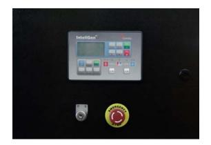
Automatic Parallel Control Panel This new automatic parallel system adopts intelligent modules, inserted and folded installed, no need the peripheral relay and logic circuit. The main switch adopts electronic breaker or frame breaker, combined together with the generator, which is very reliable. One generator, one panel. The panel can be used both for singly and parallel. It is only need to parallel generator with such panel when the capability needs to be enlarged in the future.
